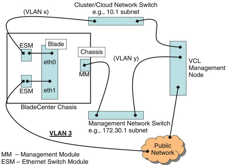
**Fig. 11.9** Undifferentiated general resource node network configuration
