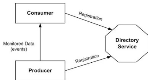
**Fig. 8.4** Grid Monitoring Architecture components
