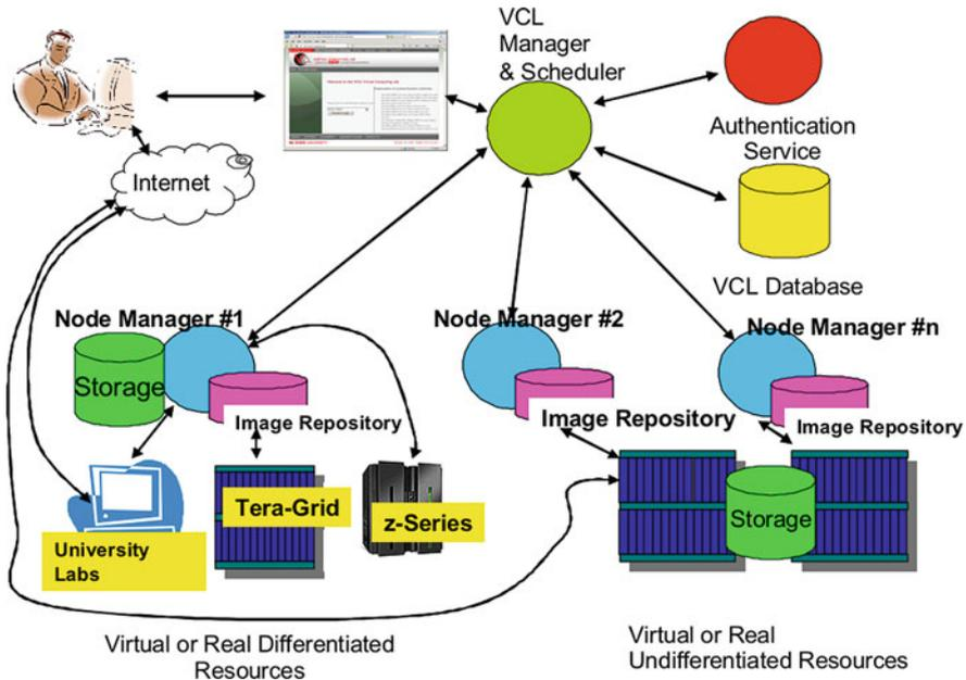
Fig. 11.5 Top level VCL architecture (Vouk et al., 2009)
