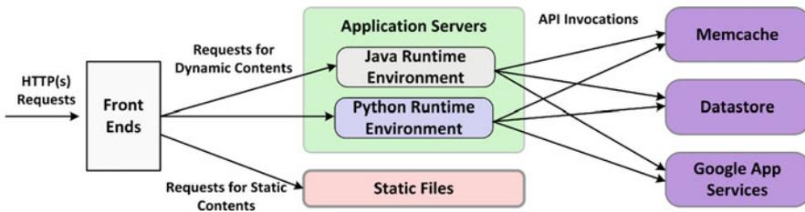
**Fig. 14.5** The Architecture of Google App Engine
