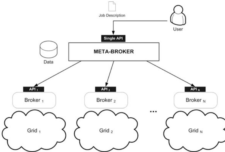
Fig. 8.6 Meta-brokering architecture
