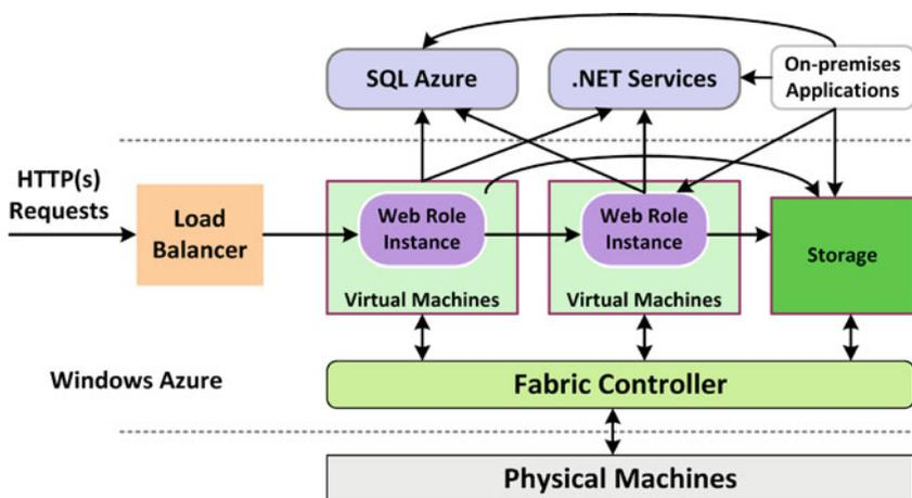
**Fig. 14.6** The architecture of the windows azure platform
