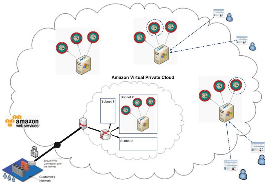
Fig. 19.7 Decentralized collaboration: Elastic-R portal as an EC2 AMI
