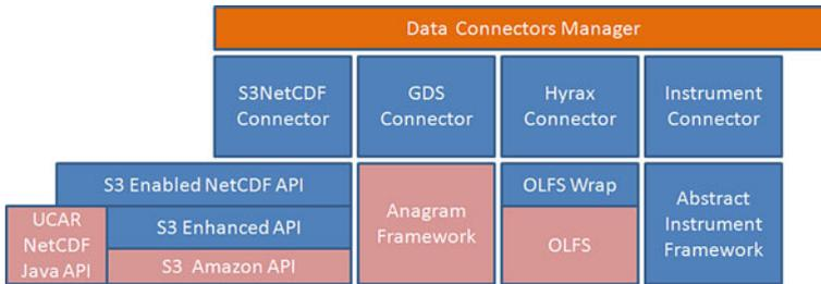
**Fig. 26.4** The NetCDF service data connector architecture
