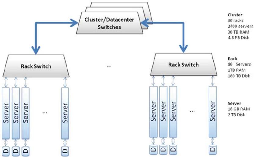
Fig. 15.2 Warehouse-scale system architecture (Barroso & Hölzle, 2009)
