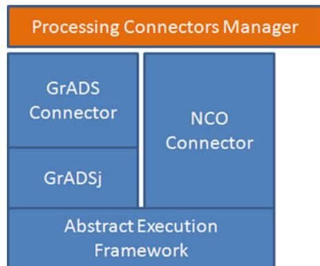
**Fig. 26.5** The NetCDF service processing connector architecture
