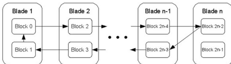
Fig. 16.6 Round robin SVD block communication pattern
