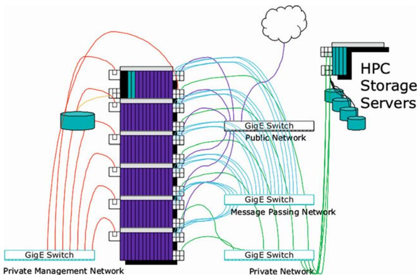
Fig. 11.13 Scalable HPC configuration
