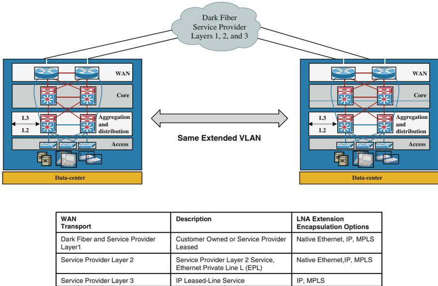
Fig. 4.3 Data center interconnect LAN extension encapsulation options
