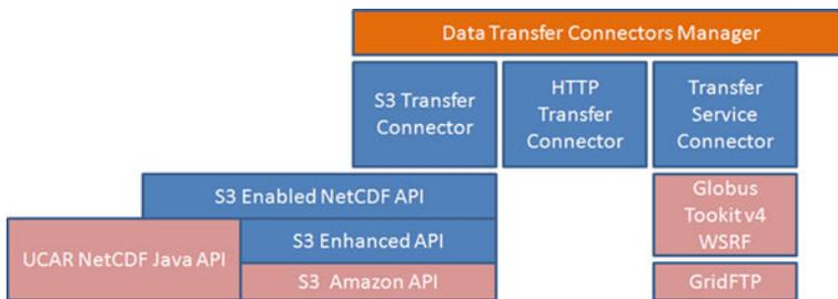
**Fig. 26.6** The NetCDF service transfer connector architecture
