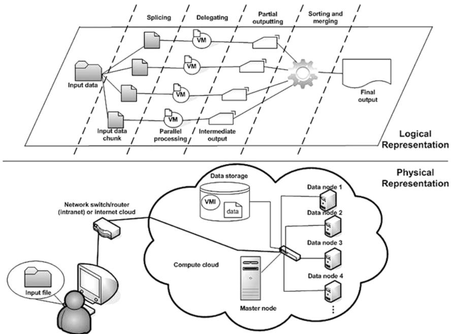
Fig. 23.3 Processing data-intensive scientific task in the cloud
