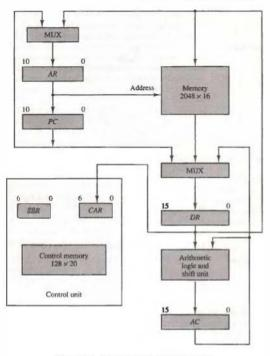
Figure 7-4 Computer hardware configuration.
