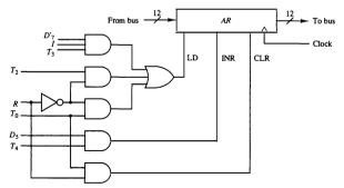
Figure 5-16 Control gates associated with AR.
