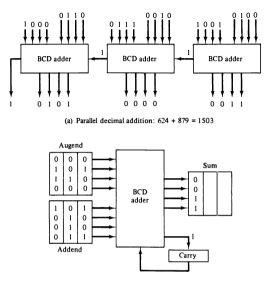
(b) Digit-serial, bit-parallel decimal addition
