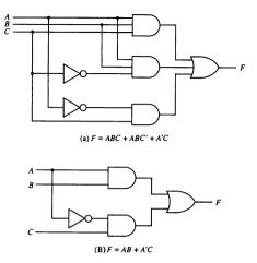
Figure 1-6 Two logic diagrams for the same Boolean function.
