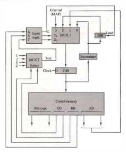
Figure 7.8 Microprogram sequencer for a concrol memory.
