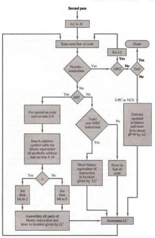
Figure 6-2 Flowchart for second pass of assembler.
