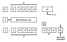
Figure 10-21 Registers for decimal arithmetic multiplication and division.
