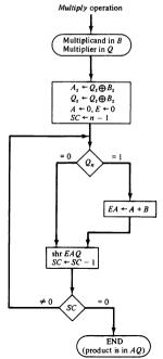
correspond to the sign of the product since a double-length product will be stored in registers A and Q. Registers A and E are cleared and the sequence counter SC is set to a number equal to the number of bits of the multiplier. We are assuming here that operands are transferred to registers from a memory unit that has words of n bits. Since an operand must be stored with its sign, one bit of the word will be occupied by the sign and the magnitude will consist of n - 1 bits.
