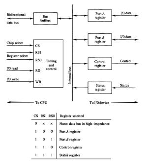
Figure 11-2 Example of I/O interface unit.
