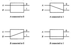
Figure 13-6 Operation of a  $2 \times 2$  interchange switch.
