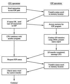
Figure 11-20 CPU-IOP communication.
