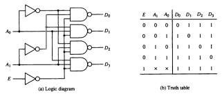
When the circuit is disabled, none of the outputs are selected and all outputs are equal to 1. In general, a decoder may operate with complemented or uncomplemented outputs. The enable input may be activated with a 0 or with a 1 signal level. Some decoders have two or more enable inputs that must satisfy a given logic condition in order to enable the circuit.
