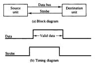
Figure 11-4 Destination-initiated strobe for data transfer.
