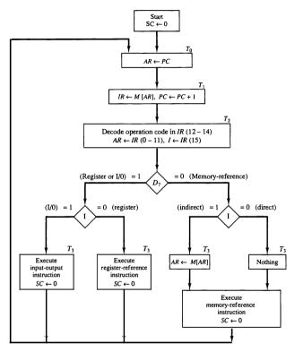
Figure 5-9 Flowchart for instruction cycle (initial configuration).
