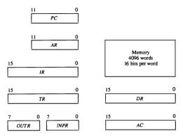
Figure 5-3 Basic computer registers and memory.
