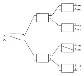
Figure 13-7 Binary tree with  $2 \times 2$  switches.
