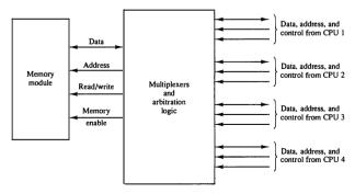
address, and control from one CPU for communication with the memc module. Priority levels are established by the arbitration logic to select one CI when two or more CPUs attempt to access the same memory. The multiplex are controlled with the binary code that is generated by a priority encoc within the arbitration logic.
