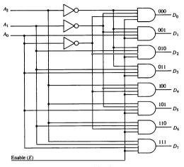
Figure 2-1 3-to-8-line decoder.
