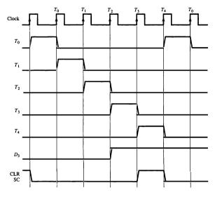
Figure 5-7 Example of control timing signals.
