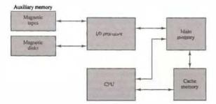
Figure 12-1 Memory hierarchy in a computer system.
