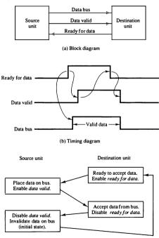
Figure 11-6 Destination-initiated transfer using handshaking.
