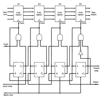
Figure 11-9 Circuit diagram of 4 × 4 FIFO buffer.
