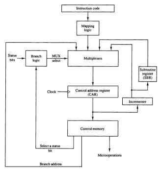
Figure 7-2 Selection of address for control memory.
