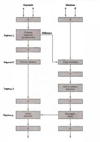
Figure 9-6 Pipeline for floating-point addition and subtraction.
