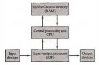
Figure 1-1 Block diagram of a digital computer.
