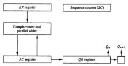
Figure 10-7 Hardware for Booth algorithm.
