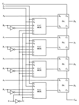
Figure 4-9 4-bit arithmetic circuit.
