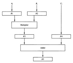
Figure 9-2 Example of pipeline processing.
