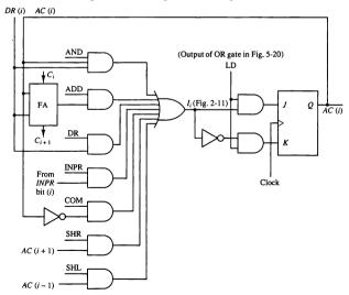
Figure 5-21 One stage of adder and logic circuit.
