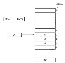
Figure 8-3 Block diagram of a 64-word stack.
