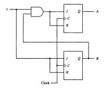
Figure 1-29 Logic diagram of a 2-bit binary counter.
