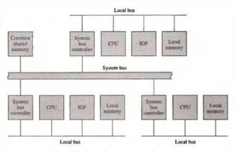
Figure 13-2 System bus structure for multiprocessors.
