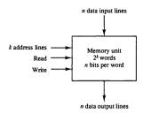
Figure 2-12 Block diagram of random access memory (RAM).
