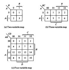
Figure 1-7 Maps for two-, three-, and four-variable functions.
