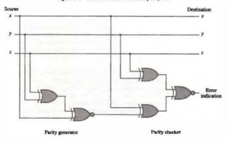
Figure 3-3 Error detection with odd parity bit.
