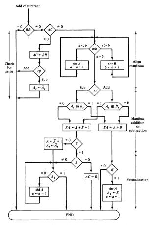
Figure 10-15 Addition and subtraction of floating-point numbers.
