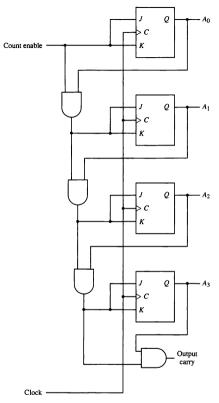
Figure 2-10 4-bit synchronous binary counter.
