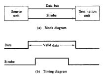
Figure 11-3 Source-initiated strobe for data transfer.
