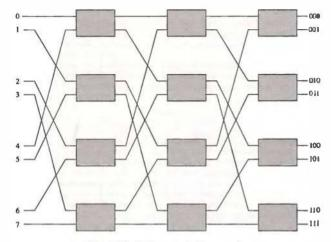
Figure 13-8 8 × 8 omega switching network.
