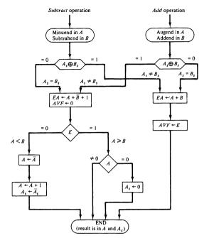
Figure 10-2 Flowchart for add and subtract operations.
