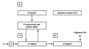
Figure 10-5 Hardware for multiply operation.
