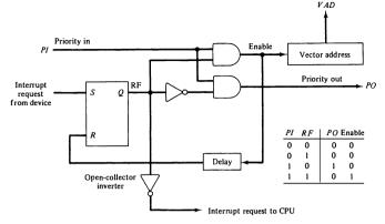
Figure 11-13 One stage of the daisy-chain priority arrangement.
