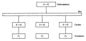
Figure 13-12 Cache configuration after a load on X.
