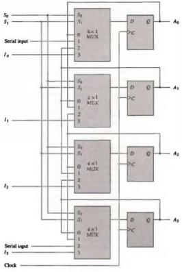
Figure 2-9 Bidirectional shift register with parallel load.
