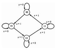
Figure 1-27 State diagram for binary counter.
