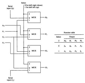
Figure 4-12 4-bit combinational circuit shifter.
