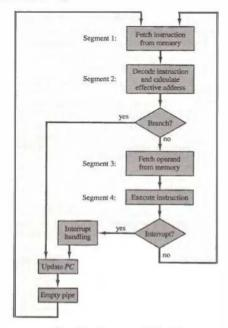
Figure 9-7 Four-segment CPU pipeline.
