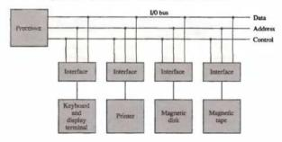
Figure 11.1 Connection of VO bus to input-output devices.
