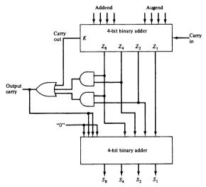
A decimal parallel-adder that adds *n* decimal digits needs *n* BCD adder stages with the output-carry from one stage connected to the input-carry of the next-higher-order stage. To achieve shorter propagation delays, BCD adders include the necessary circuits for carry look-ahead. Furthermore, the adder circuit for the correction does not need all four full-adders, and this circuit can be optimized.
