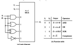
Figure 4-10 One stage of logic circuit.
