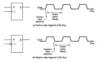
Figure 1-23 Edge-triggered flip-flop.
