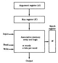
specifies how the reference to memory is made. To illustrate with a numerical example, suppose that the argument register A and the key register K have the bit configuration shown below. Only the three leftmost bits of A are compared with memory words because K has 1's in these positions.
