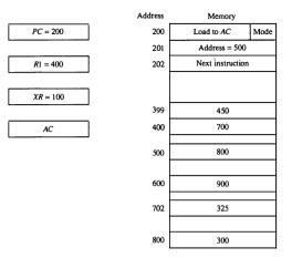
Figure 8-7 Numerical example for addressing modes.
