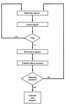
Figure 11-11 Flowchart for CPU program to input data.
