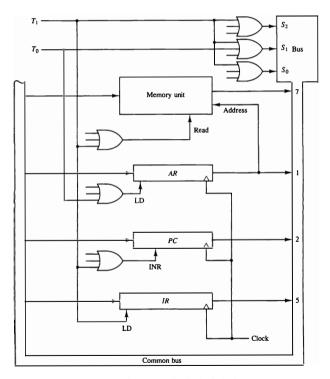
Figure 5-8 Register transfers for the fetch phase.
