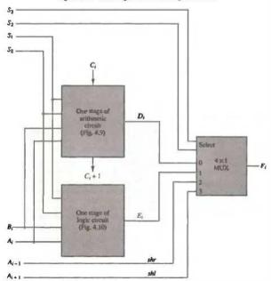
Figure 4-13 One stage of arithmetic logic shift unit.
