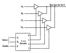
Figure 4-5 Bus line with three state-buffers.
