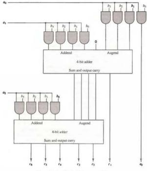
Figure 10.10 4-bit by 3-bit array multiplier.
