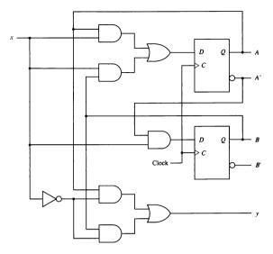
Figure 1-25 Example of a sequential circuit.
