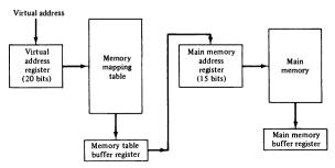
Figure 12-17 Memory table for mapping a virtual address.
