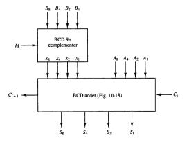
Figure 10-19 One stage of a decimal arithmetic unit.
