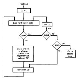
Figure 6-1 Flowchart for first pass of assembler.
