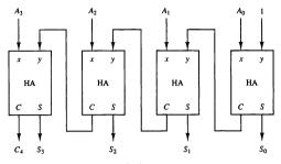
Figure 4-8 4-bit binary incrementer.
