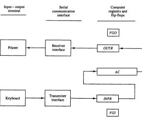
Figure 5-12 Input-output configuration.
