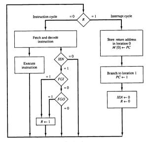
Figure 5-13 Flowchart for interrupt cycle.
