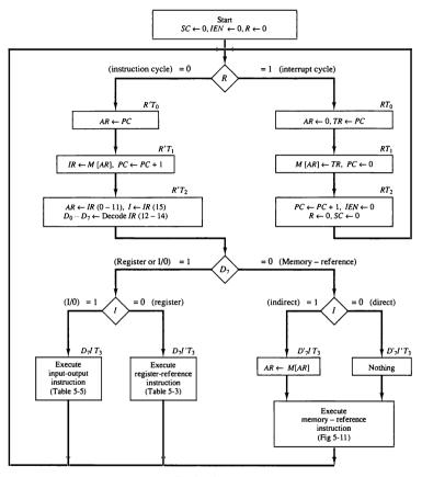
Figure 5-15 Flowchart for computer operation.
