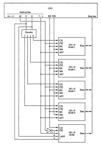
Figure 12-4 Memory connection to the CPU.
