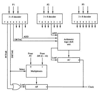
Figure 7-7 Decoding of microoperation fields.
