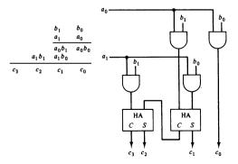
Figure 10-9 2-bit by 2-bit array multiplier.
