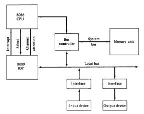
Figure 11-23 Intel 8086/8089 microcomputer system block diagram.
