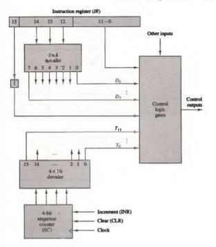
Figure 5-6 Control unit of basic computer.
