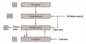
Figure 10.1 Hardware for signed-magnitude addition and subtraction.
